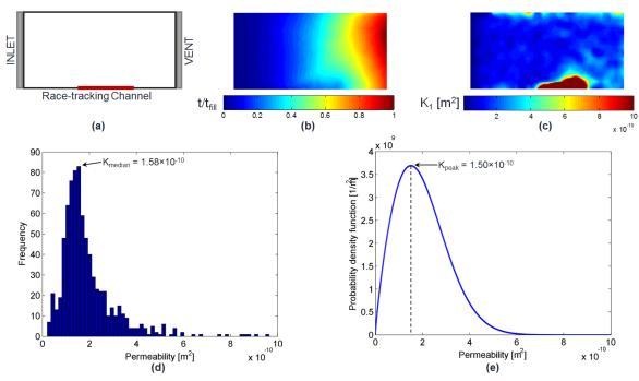
**Figure 2:** Results of an experiment with a race-tracking channel introduced intentionally. (a) Mold details, (b) flow front propagation in the experiment, (c) estimated permeability map, (d) histogram of the estimated permeability values, (e) probability density function corresponding to the histogram.
