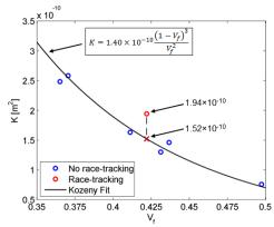
Figure 1: Results of one-dimensional rectilinear permeability experiments.
